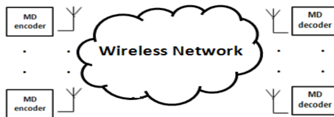
Figure 4: Transmitter and receiver structure.
