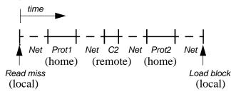
Figure 2: Timing of a read miss to a dirty memory block.
