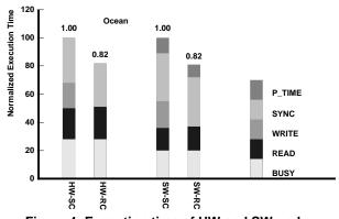
Figure 4: Execution time of HW and SW under sequential consistency (SC) and release consistency (RC) in Ocean. The execution time is normalized for each system to the execution time under sequential consistency.
